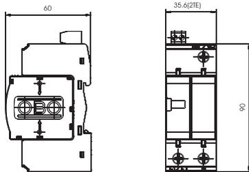
Application: lightning protection equipotential bonding in buildings which also have external lightning protection of Classes III and IV and in standard distributor housings.
