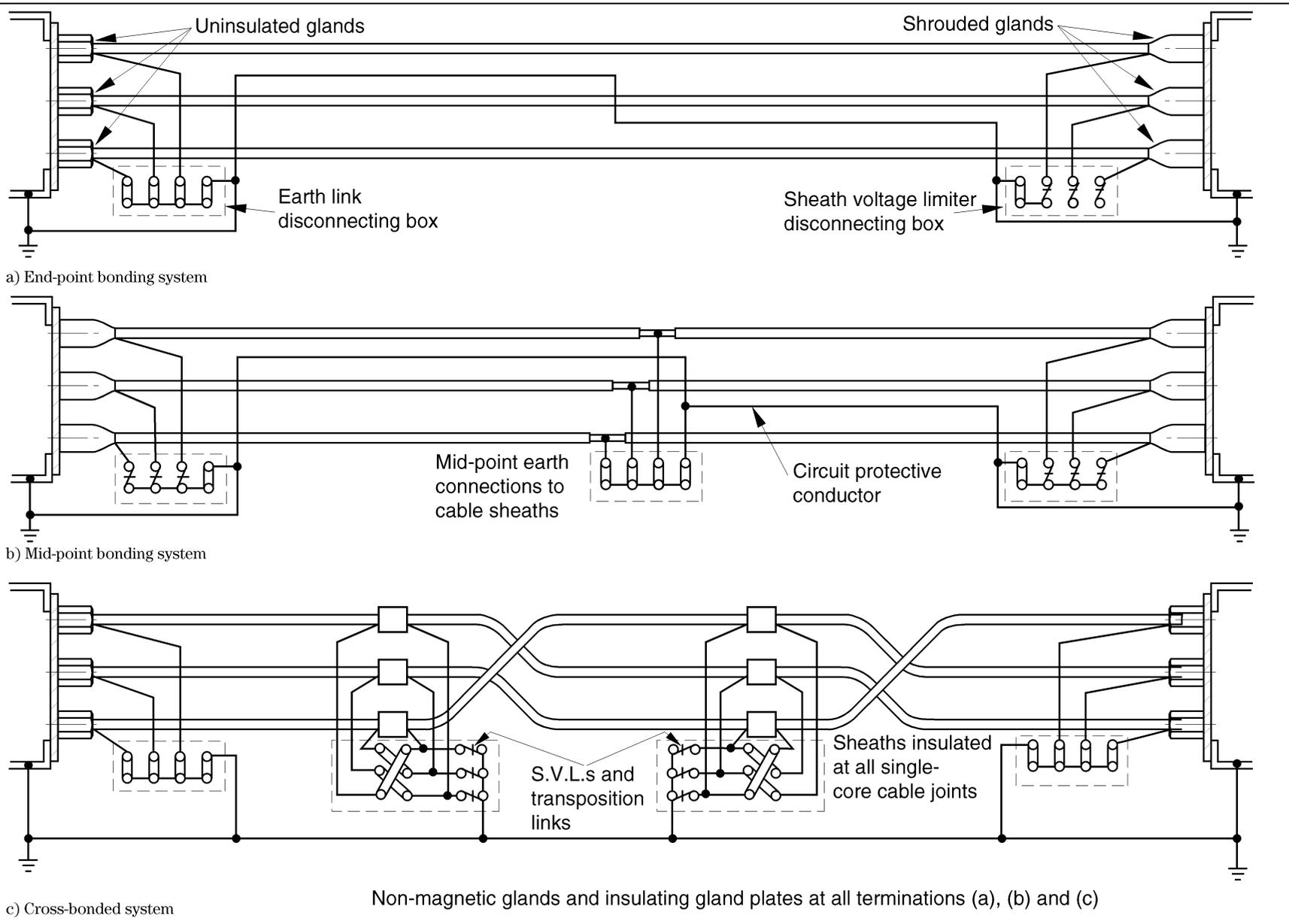
Figure 23 — Simplified illustration of single-core cable sheath bonding systems
