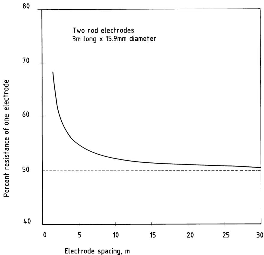
Figure 4 — Effect of inter-electrode spacing on combined resistance
