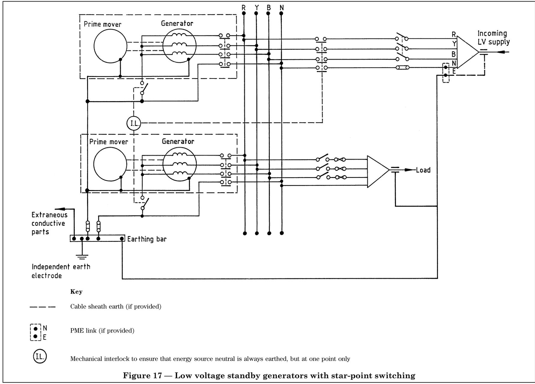
Figure 17 — Low voltage standby generators with star-point switching
