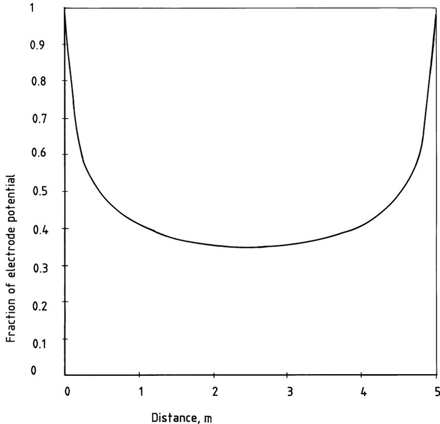
Figure 10 — Potential distribution between rod electrodes
