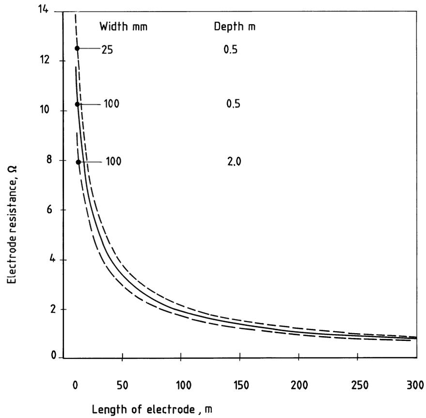
Figure 6 — Resistance of horizontal strip electrodes
