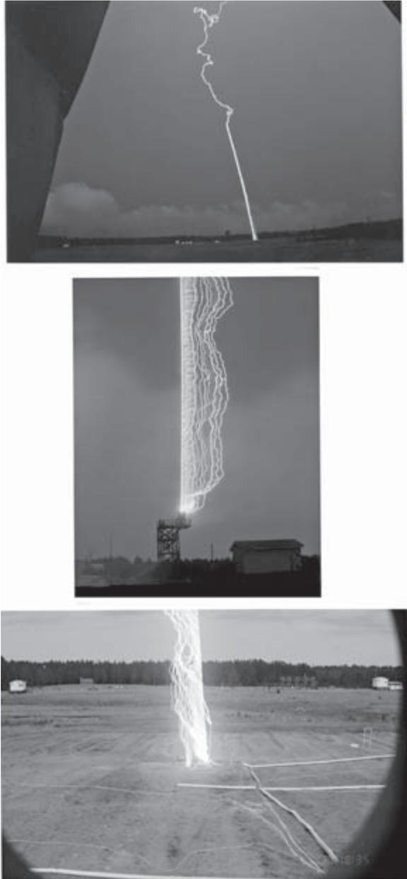
Figure 3.2 Photographs of lightning flashes triggered at Camp Blanding, Florida. Top, a distant view of a strike to the test runway; middle, a strike to the test power system initiated from the tower launcher; bottom, a strike initiated from the underground launcher at the centre of a  $70 \times 70 \text{ m}^2$  buried metallic grid.
