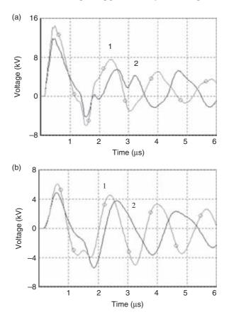
Figure 12.33 Induced voltages at the transformer LV terminals for the bunched cable versus open wire line configuration: (a) phase-to-earth; (b) phase-to-neutral. Curve 1, open wire line; curve 2, bunched cable.
