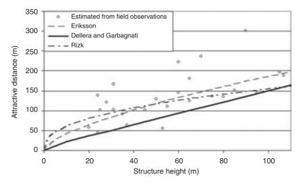
Figure 4.30 Lateral attractive distance estimated from field observations [59] and predicted by the Eriksson [58,59], Dellera and Garbagnati [28,60] and Rizk [96,98] models for free-standing structures as a function of height. A prospective return stroke peak current of 31 kA was assumed for the models.
