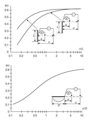
Figure 6.34 Correct ratio of voltage probe distance b = TP and current electrode distance c = TA as function of the dimensions of a long strip earth-electrode [20-22]
