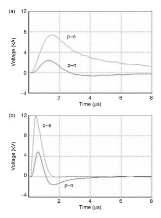
Figure 12.18 Phase-to-earth (p-e) and phase-to-neutral (p-n) induced voltages in the middle of the line for the situation indicated in Figure 12.16 and stroke currents shown in Figure 12.17a: (a) first stroke; (b) subsequent stroke
