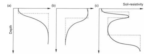
Figure 15.11 Adaptation of earth electrode design to the soil resistivity configuration: (a) low-resistivity topsoil over high-resistivity subsoil; (b) high-resistivity topsoil over low-resistivity subsoil; (c) topsoil and subsoil strata alternately of low and high resistivity. Continuous line, measured resistance; dashed line, deduced stratification.
