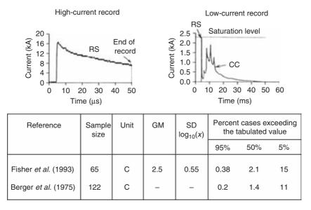
Figure 3.9 Total stroke charge. RS is the return stroke, CC is the continuing current, GM the geometric mean and SD the standard deviation of the logarithm (base 10) of the parameter (adapted from Reference 68).
