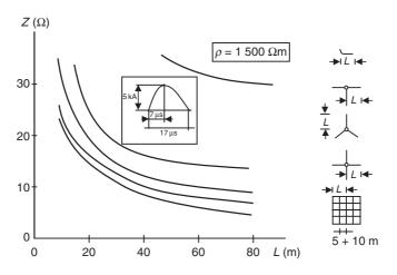
Figure 6.22 Conventional earth resistance of various earth-termination systems
