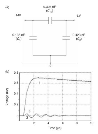
Figure 12.40 Equivalent capacitive PI-circuit and comparison of measured and calculated phase-to-neutral voltages transferred to the secondary of the 30 kVA transformer, in the no-load condition, for a standard 1.2/50 µs impulse voltage of 1.7 kV applied to the primary terminals short-circuited: (a) equivalent capacitive PI-circuit; (b) transferred voltages (curve 1, capacitive PI-circuit; curve 2, model indicated in Figure 12.6; curve 3, measured)
