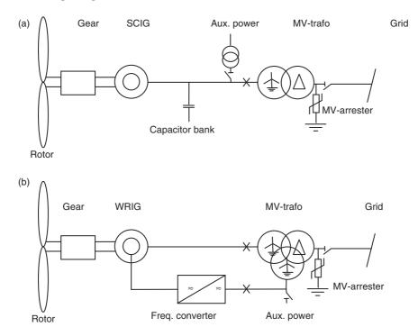
Figure 14.20 Two typical electrical system configurations in wind turbines. (a) An asynchronous squirrel cage induction generator (SCIG) with capacitor bank for phase compensation and two winding machine transformer. (b) A wound rotor induction generator (WRIG) with a frequency converter in the rotor circuit and three-winding machine transformer.
