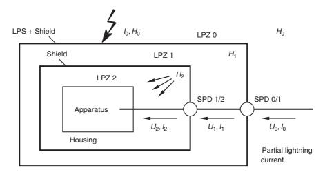
Figure 21.9 Example of a structure with a LEMP protection measures system (LPMS)
