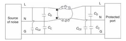
Figure 5.17 A general power supply filter
