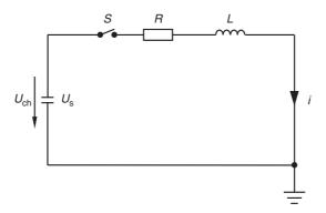
Figure 22.11 Equivalent R-L-C circuit of a high-current generator
