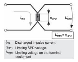
Figure 7.55 Connection of SPDs in serial connection
