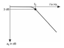
Figure 7.83 Typical frequency response of a BLITZDUCTOR CT
