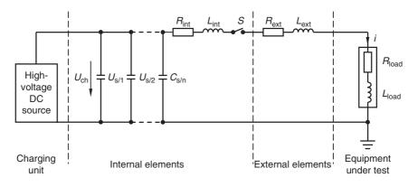
Figure 22.9 High-current impulse generator
