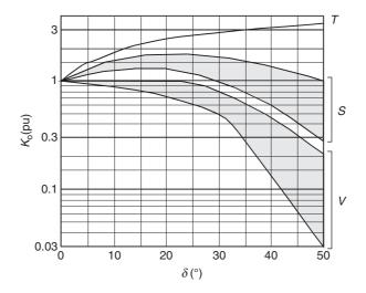
Figure 13.1 Direct strikes to an MV line. Orography correction coefficient K<sub>o</sub> as a function of the orography parameters defined in Figure 13.2 (adapted from Reference 19).
