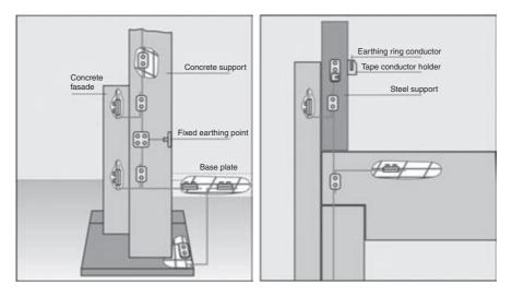
Figure 7.16 Shielding of a structure or building
