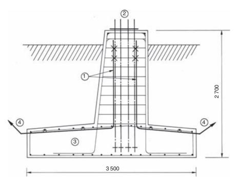
Figure 15.18 Bonding of the tower feet to reinforcement bars in the concrete foundations and to the soil or rock beneath: galvanized-steel strips (about  $30 \times 3 \text{ mm}^2$ , 1), welded to the feet of two diagonally opposed tower corner elements (2) and welded or clamped to the reinforcement bars in the concrete foundation (3) and extended (4) to connect to the buried earth system. Typical dimensions are shone in mm.
