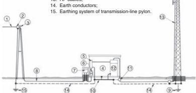
Figure 15.7 Elements of a low-power television and VHF/FM rebroadcasting station, such as that depicted in Figure 15.6
