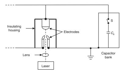
Figure 22.19 Laser-triggered crowbar spark gap
