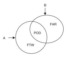
Figure 19.14 Venn diagram depicting a single-stage lightning warning system. B is the set of warning actions and A is the set of lightning occurrences. The probabilities for each of the three interior regions (members of the two set) are FAR, POD and FTW, as discussed in Section 19.4.
