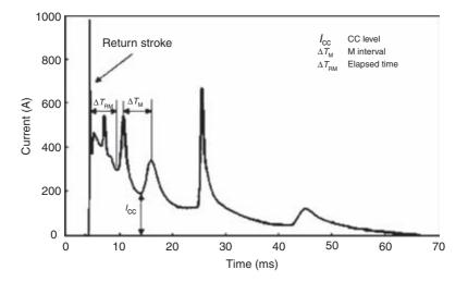
Figure 2.40 A current record showing one return stroke followed by several M-components ( $I_{CC}$ , continuing current level;  $\Delta T_M$ , M-interval;  $\Delta T_{RM}$ , elapsed time) (from Reference 133)
