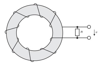
Figure 22.30 Principle of a current monitor
