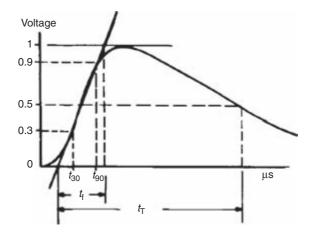
*Figure 13.5 Standard lightning impulse waveshape (adapted from Reference 3)*
