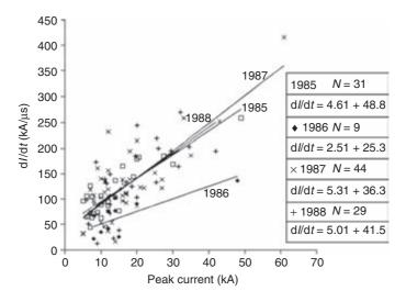
Figure 3.8 Relation between peak current rate of rise, dI/dt, and peak current I, from triggered-lightning experiments conducted at the NASA Kennedy Space Center, Florida, in 1985, 1987 and 1988 and in France in 1986. The regression line for each year is shown, and the sample size and the regression equation are given (adapted from Reference 71).
