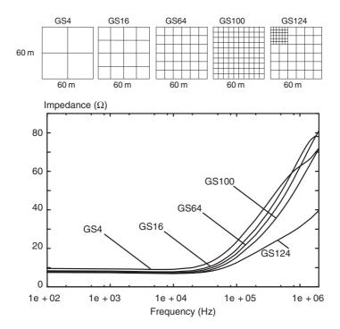
Figure 10.16 Influence of conductor separation on harmonic impedance
