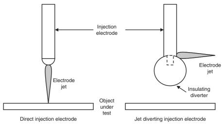
Figure 22.25 Types of injection electrodes
