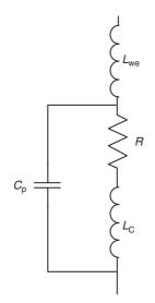
Figure 5.24 Possible equivalent circuit of a resistor
