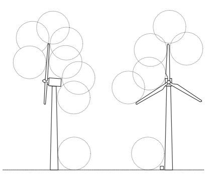
Figure 14.10 Application of the rolling sphere method for identifying lightning protection zones  $0_A$  in which lightning can attach and  $0_B$  which lightning cannot reach. A transformer cubicle next to the tower can be placed within lightning protection zone  $0_B$ .
