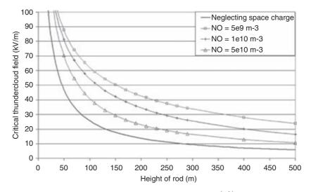
Figure 4.21 Critical thundercloud electric field  $E_{cloud}^{(crit)}$  required to initiate upward leaders as a function of the tower height, for different initial aerosol particle concentrations:  $5 \times 10^9 \text{ m}^{-3}$  (squares),  $1 \times 10^{10} \text{ m}^{-3}$  (crosses),  $5 \times 10^{10} \text{ m}^{-3}$  (triangles). The critical leader inception electric field computed by neglecting the space charge layer is also shown (line with no symbols).
