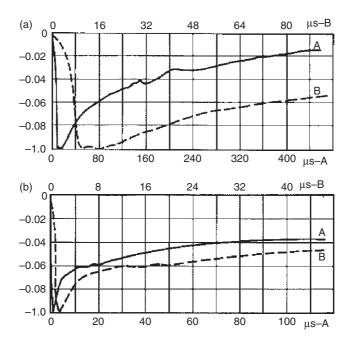
Figure 2.27 The mean current wave shapes of (a) first and (b) subsequent returnstroke current waveforms based on the experimental data of Berger et al. [98]
