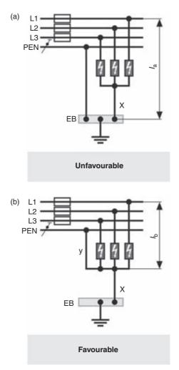
Figure 7.60 (a) Unfavourable connection of SPDs with consideration of the recommended maximum cable lengths. (b) Favourable connection of SPDs with consideration of the recommended maximum cable lengths.
