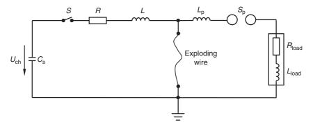
Figure 22.22 Impulse current generator with exploding wire
