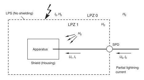
Figure 21.8 Example of a structure with LPS according to IEC 62305-3 (Section 21.4)
