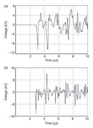
Figure 12.37 Phase-to-neutral transferred voltages at the transformer LV terminals: (a) first stroke; (b) subsequent stroke. The lightning strike point is 800 m from the transformer. Stroke current waveforms are depicted in Figure 12.17a.
