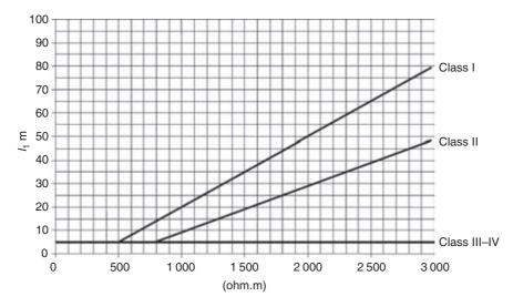
Figure 15.17 Minimum lengths  $l_1$  of each earth-electrode according to the class of LPS
