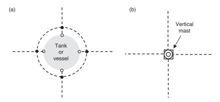
Figure 17.2 (a) The grounding system (top view) for a tank or vessel. Points at which the grounding system is bonded to the tank are marked by empty circles. The vertical ground rods are marked by full circles. The ground conductor buried at a depth of at least 0.6 m is marked by a dashed line. (b) The vertical mast (top view) should have multiple paths for lightning current near the connecting point in order to reduce potential rise [13].
