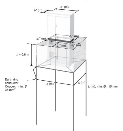
Figure 6.27 Practical earth-termination system of a shelter in reduced space
