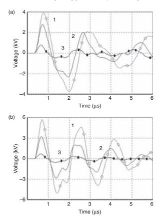
Figure 12.29 Phase-to-neutral induced voltages at the entrance of the closest consumer to the stroke location for the configuration shown in Figure 12.23: (a) height of neutral conductor: 6.48 m; (b) height of neutral conductor: 7.0 m. Low-voltage power installations represented as inductances (L) of different values. Curve 1,  $L = 20 \mu H$ ; curve 2,  $L = 10 \mu H$ ; curve 3,  $L = 2 \mu H$ .
