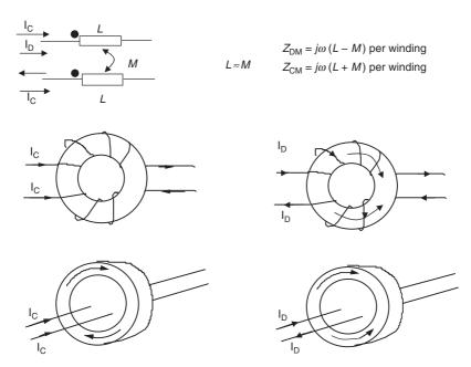
Figure 5.15 Differential- and common-mode operation of chokes
