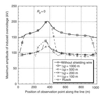
Figure 13.12 Maximum amplitude of the induced voltage along the line as a function of the spacing ( $\Delta g$ ) between two adjacent groundings of the shielding wire. Line configuration of Figure 13.11, stroke location 50 m from the line and 370 m from left line termination. Perfectly conducting ground. Lightning current: maximum amplitude 30 kA maximum time derivative 100 kA  $\mu s^{-1}$  (adapted from Reference 32).
