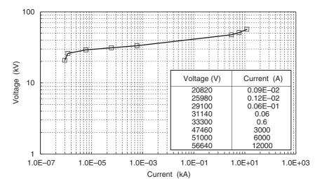
*Figure 13.14* Surge arrester V–I characteristic (adapted from Reference 32)
