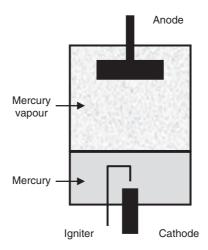
Figure 22.18 Functional principle of an ignitron
