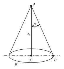
Figure 6.6 Volume protected by a vertical air-termination rod. A is the tip of the airtermination rod, B is the reference plane, OC is the radius of the protected area, and  $h_1$  is the height of the air-termination rod above the reference plane of protection.
