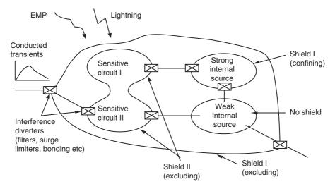
Figure 5.3 A two-layer shielding topology and the role of surge protection
