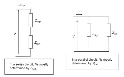
Figure 5.22 Series and parallel circuits
