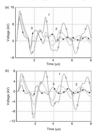
Figure 12.28 Induced voltages at the transformer LV terminals for different transformer models: (a) phase-to-earth; (b) phase-to-neutral. Curve 1,  $L = 40 \ \mu$ H; curve 2, parallel RLC circuit ( $R = 367 \ \Omega$ ,  $L = 16 \ \mu$ H,  $C = 2.28 \ n$ F) – base case; curve 3, parallel RLC circuit ( $R = 253 \ \Omega$ ,  $L = 4.1 \ \mu$ H,  $C = 3 \ n$ F).
