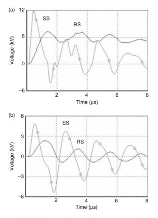
Figure 12.20 Induced voltages at the transformer LV terminals for the first (RS) and subsequent (SS) stroke currents shown in Figure 12.17. Line configuration indicated in Figure 12.19 (a) phase-to-earth (b) phase-to-neutral.
