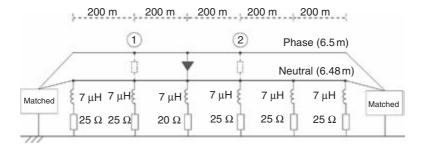
Figure 12.31 Low-voltage line configuration for the induced voltages shown in Figure 12.32 (side view). The triangle and the dotted rectangles denote, respectively, the secondary of the distribution transformer and LV power installations.
