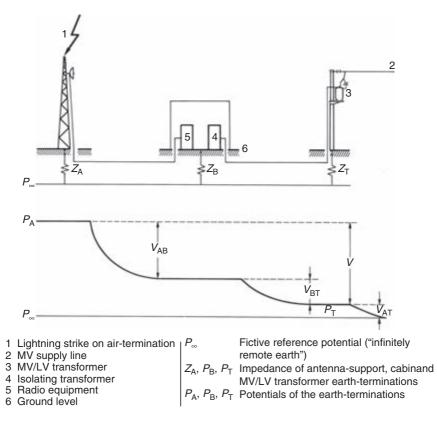
*Figure 15.4 Typical earth potential pattern during a lightning flash to a station having three separate earth-terminations*
