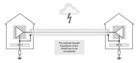
*Figure 7.19 Shield connection at both ends: shielding from capacitive/inductive couplings*
