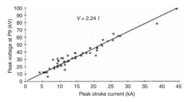
Figure 3.27 Peak induced voltage (8 to 100 kV) at pole 9 versus return-stroke peak current (4 to 44 kA), n = 63 (adapted from Reference 98)
