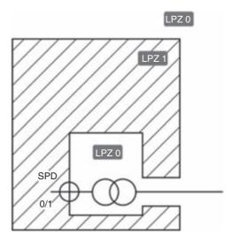
Figure 7.29 Transformer inside the structure or building (LPZ 0 integrated in LPZ 1)
