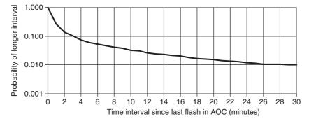
Figure 19.7 Cumulative distribution of the time interval between successive flashes in a  $10 \times 10$  km<sup>2</sup> AOC centred on the Pittsburgh International Airport in the United States. Eight years of NLDN data were used to produce the analysis.
