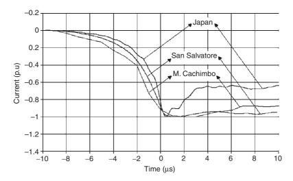
Figure 2.28 The mean curve representing the first 10  $\mu$ s of the first return-stroke current waveform. The peak current is normalized to unity.
