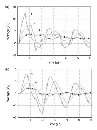
Figure 12.21 Induced voltages at the transformer LV terminals corresponding to stroke currents with triangular waveforms and various front times (tf): (a) phase-to-earth (b) phase-to-neutral. Line configuration indicated in Figure 12.19. Curve 1, tf = 0.5  $\mu$ s; curve 2, tf = 1  $\mu$ s; curve 3, tf = 2  $\mu$ s.
