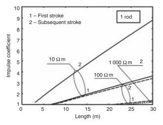
Figure 10.19 Impulse coefficient of a single vertical rod
