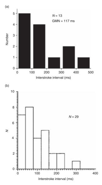
Figure 2.9 Interstroke interval of positive ground flashes as observed in (a) Brazil [31] and (b) Sweden (from Reference 28)
