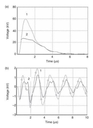
Figure 12.42 Phase-to-neutral voltages at the transformer terminals considering the typical subsequent stroke current depicted in Figure 12.17a: (a) induced voltages at the MV side; (b) transferred voltages to the LV side. Curve 1, without MV surge arresters; curve 2, with MV surge arresters.
