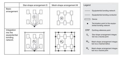
Figure 7.25 Integration of electronic systems into the equipotential bonding network
