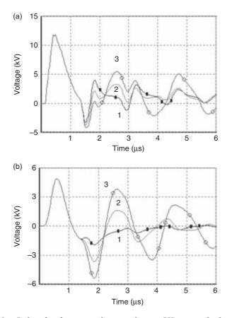
Figure 12.32 Induced voltages at the transformer LV terminals for a different number of LV power installations connected to the line, according to the configuration shown in Figure 12.31: (a) phase-to-earth; (b) phase-to-neutral. Curve 1, all power installations disconnected from the line; curve 2, just one power installation connected to the line, at point 1; curve 3, two power installations connected to the line, at points 1 and 2.
