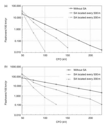
Figure 13.23 Line flashover rate curves obtained by using LIOV–MC for the case of a line with and without surge arresters located every 200 and 500 m: (a) ideal ground and (b) lossy ground ( $\sigma_{g \ 0.01} = 1 \text{ mS m}^{-1}$ ) (adapted from Reference 54).
