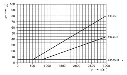
Figure 21.6 Reference length  $l_1$  of an earth electrode as a function of soil resistivity  $\rho$
