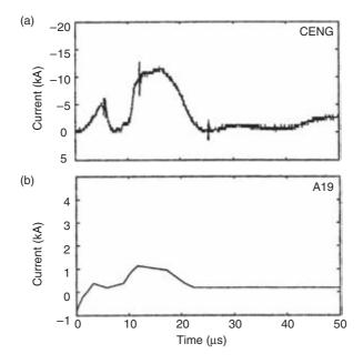
Figure 3.28 Current versus time waveforms for flash 9516, displayed on a 50  $\mu$ s scale: (a) total lightning current, CENG; (b) ground-rod current, A19, measured 60 m from the lightning strike point (adapted from Reference 46)
