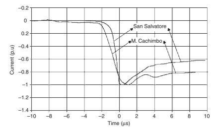
Figure 2.29 The mean curve representing the first  $10 \ \mu s$  of the subsequent returnstroke current waveform. The peak current is normalized to unity.
