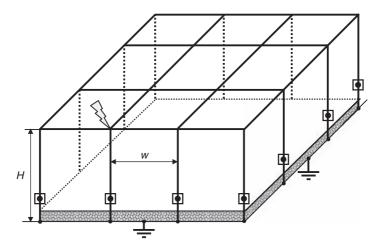
Figure 6.19 Partitioning coefficient  $k_c$  in the case of a meshed air-termination system and a type B earth-termination system.  $k_c = 1/2n + 0.1 + 0.2 \times \sqrt[3]{(W/H)}$ , where n is the total number of down-conductors (add internal down-conductors if they exist), w the spacing between down-conductors and H the height (spacing) between horizontal ring conductors.
