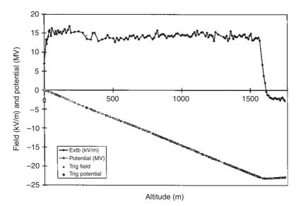
Figure 2.4 Ambient electrostatic field (upper trace) and potential profile (lower trace) as a function of height (from Reference 5)
