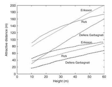
Figure 4.29 Comparison of the attractive distance of a free-standing structure predicted by the Eriksson [58,59], Dellera and Garbagnati [28,60] and Rizk models [96,98] for prospective return stroke peak currents of 60 kA (solid lines) and 20 kA (dashed lines) (adapted from Reference 99)
