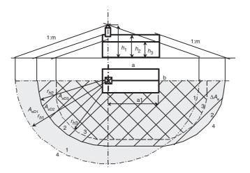
Figure 8.4 Collection area boundaries for different parts of a structure with complex shape. 1, boundary for part with height  $h_1$ ; 2, boundary for part with height  $h_2$ ; 3, boundary for part with height  $h_3$ ; 4, resulting boundary.
