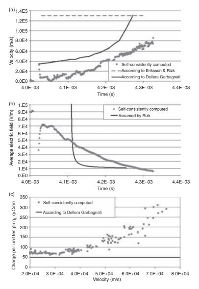
Figure 4.33 Comparison between the upward connecting leader parameters selfconsistently computed with the model presented in Reference 104 and the values assumed by the leader progression models for the rocket-triggered experiment reported in Reference 49: (a) leader velocity, (b) average electric field along the leader channel and (c) charge per unit length of the leader as a function of its velocity (adapted from Reference 106)
