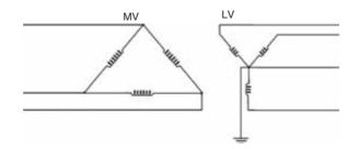
Figure 12.4 Delta–earthed wye connection
