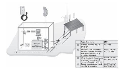
Figure 7.95 Protection concept for data acquisition and evaluation
