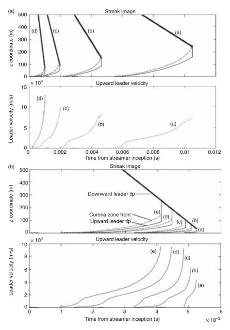
*Figure 4.34* (a) Simulated streak image and leader velocity variation of the upward connecting leader for different values of the downward leader velocity for a lightning flash with 87 kA return stroke peak current striking.
