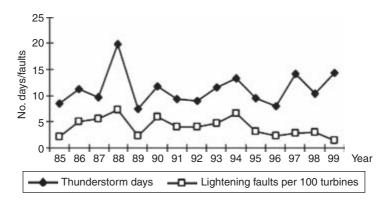
Figure 14.7 Registered lightning faults per 100 turbines in Denmark in the period 1985–1999 shown together with the registered thunderstorm days (keraunic level) (from Reference 11)
