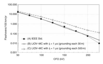
Figure 13.21 Comparison between the line flashover rate curve of IEEE Std. (A) and those obtained by using LIOV–MC, enforcing  $t_f = 1 \ \mu s$  for each event, for two different shielding wire grounding spacings, 30 m (B) and 500 m (C) (adapted from Reference 54).
