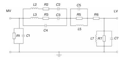
Figure 12.6 Simplified distribution transformer model for evaluation of transferred voltages (adapted from References 18 and 19)
