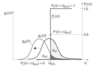
Figure 8.7 Graphical interpretation of overvoltages causing damages with probabilities  $p_{sjl}$  and  $p_{sj2}$  shown by shaded surfaces in the case of stepped damage distribution function  $P_i(U)$
