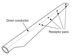
*Figure 14.16 Lightning protection for large blades with receptor pairs at the tip and on the sides of the blade*
