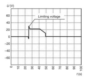
Figure 7.81 Limiting voltage at nominal discharge current
