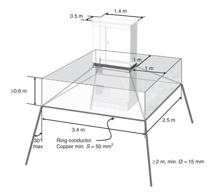
Figure 6.26 Earth-termination system of a metallic shelter
