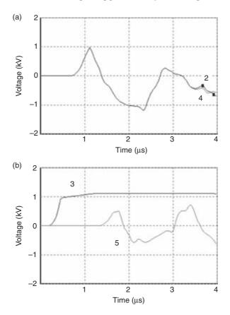
Figure 12.50 Phase-to-neutral induced voltages at points 2, 3, 4 and 5 of Figure 12.47 considering a first stroke with the current waveform depicted in Figure 12.17a but with amplitude of 88.5 kA: (a) points 2 (curve 2) and 4 (curve 4); (b) points 3 (curve 3) and 5 (curve 5). Configuration 2 (arresters only at the transformer terminals).
