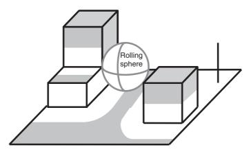
Figure 21.4 Application of the rolling sphere method to a structure to be protected
