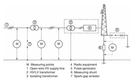
Figure A15.1 Measurement of overvoltages caused by simulated lightning flash to the antenna support
