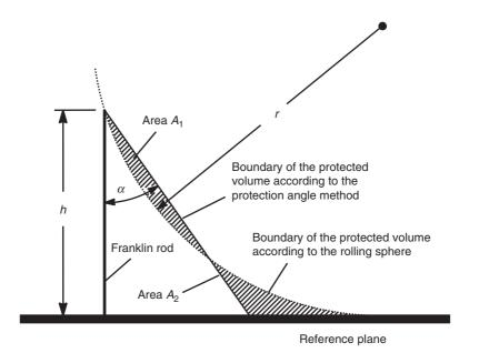
Figure 21.5 Application of the protection angle method for a Franklin rod of height h, where r is the rolling sphere radius and  $\alpha$  the protection angle
