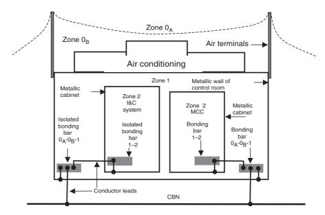
Figure 17.6 Typical lightning protection scheme for a control room containing motor control centre (MCC) and I&C devices and circuits in an OOI
