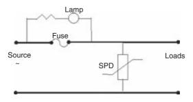
Figure 5.14 Use of a fuse in conjunction with an SPD
