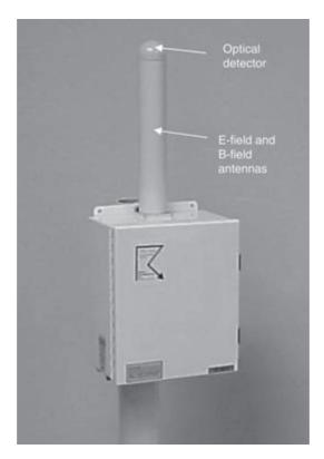
Figure 19.2 A single-point VLF–LF and optical lightning sensor. The vertical antenna assembly contains both electric and magnetic field antennas. The optical sensor sits atop the antenna assembly.
