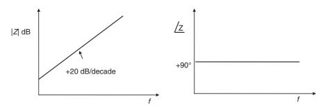
Figure 5.20 Impedance magnitude and phase of an ideal inductor
