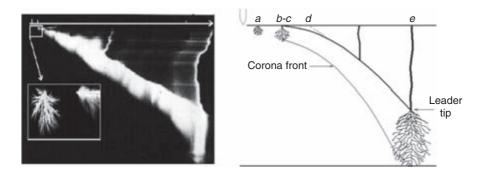
Figure 4.12 Streak image and sketch of the development of positive leaders in laboratory long air gaps (adapted from Reference 71)
