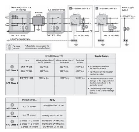
Figure 7.92 Basic circuit diagram: surge protection for a PV installation at a building with an external lightning protection system: (a) TT system 230 V a.c.; (b) TN system 230 V a.c
