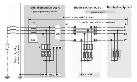
Figure 7.54 Use of SPDs in IT systems without neutral conductor
