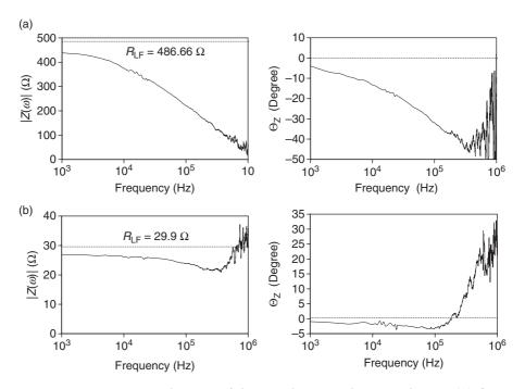
Figure 9.8 Frequency diagram of the complex grounding impedance  $Z(\omega)$  for a 12-m-long horizontal electrode. Ratio of the voltage and current phasors  $[\underline{V}(\omega)/\underline{I}(\omega)]$ : (a) high-resistivity soil (3.8 k $\Omega$ m) and (b) low-resistivity soil (250  $\Omega$ m) (adapted from Reference 7).
