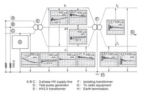
Figure A15.7 Observation of simulated overvoltages surges transferred from the supply line
