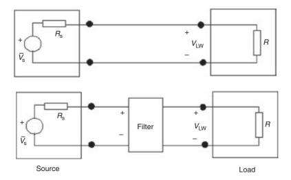
Figure 5.16 System comprising of source and load with and without filter
