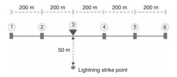
Figure 12.47 Low-voltage line configurations. The triangles and rectangles denote, respectively, the distribution transformer and the LV power installations. Configuration 1, line without arresters; configuration 2, arresters only at point 3; configuration 3, arresters at points 1, 2, 3, 5 and 6.
