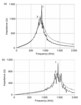
Figure 12.5 Comparison of the magnitudes of the transformer input impedance seen from each LV terminal (1) and the impedance of an RLC parallel circuit (2): (a) 30 kVA transformer ( $R = 1\,100\,\Omega$ ,  $L = 48\,\mu$ H and  $C = 0.76\,n$ F); (b) 112.5 kVA transformer ( $R = 760\,\Omega$ ,  $L = 12.4\,\mu$ H and  $C = 1.0\,n$ F)
