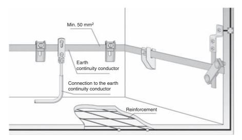
Figure 7.17 Earth continuity conductor
