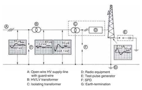
Figure A15.6 Observation of a simulated lightning strike on an antenna support
