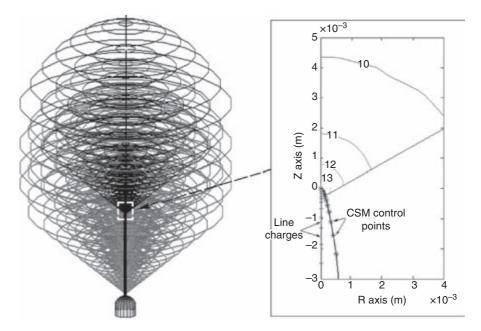
Figure 4.31 Detail of the representation of the leader channel tip and the specific power in the corona zone in the self-consistent leader progression model of Becerra and Cooray [104]. The contours correspond to the logarithm of the specific power evaluated taking into account the effect of space charge produced during previous steps.
