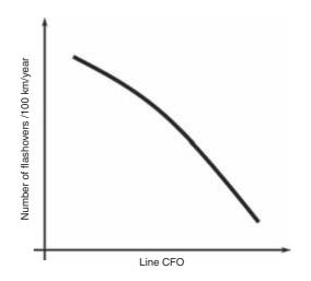
Figure 13.18 Lightning performance of a distribution line
