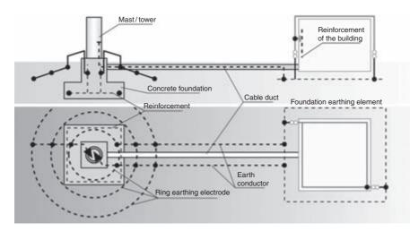
Figure 7.86 Intermeshed network of earthing electrodes of a wind turbine
