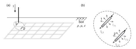
Figure 9.2 Elements of a grounding system: (a) the whole grounding system; (b) two elements taken from the grounding system (adapted from Reference 2)
