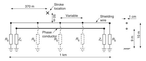
Figure 13.11 Configuration adopted to evaluate the mitigation effect of shielding wires on lightning-induced voltages. Lightning current: maximum amplitude 30 kA maximum time derivative 100 kA  $\mu s^{-1}$  (adapted from Reference 32).
