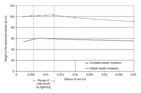
Figure 4.25 Height of the downward leader tip where unstable and stable upward leader inception takes place from a 10-m-high rod as function of its radius. The downward stepped leader is assumed to have a prospective return stroke peak current of 10 kA and an average velocity of  $5 \times 10^5$  m s<sup>-1</sup> [73]. The range of radii of the blunt lightning rods struck by lightning in the experiment of Moore and colleagues [87,88] is also shown.
