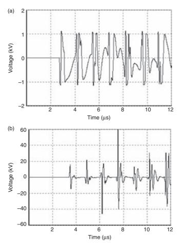
Figure 12.53 Phase-to-neutral transferred voltages at points 3 and 4 of Figure 12.47, considering the typical subsequent stroke current depicted in Figure 12.17a: (a) point 3 (transformer); (b) point 4. The strike point is 800 m from the transformer. Configuration 2 (arresters only at the transformer terminals).
