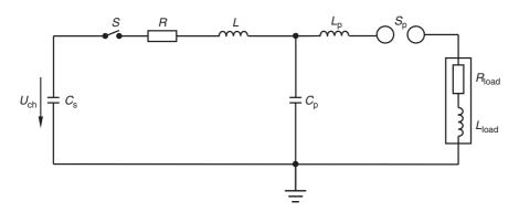
Figure 22.20 Impulse current generator with peaking circuit
