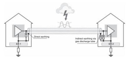
Figure 7.20 Shield connection at both ends preventing equalizing currents: direct and indirect shield earthing
