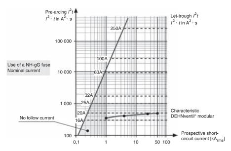
Figure 7.75 Disconnection selectivity of DEHNventil modular to NH fuse holders with different rated currents
