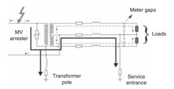
Figure 12.45 Injection of current into the neutral due to a direct strike to the MV line
