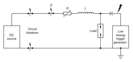
Figure 22.24 Basic circuit of a long-duration generator for a rectangular waveform
