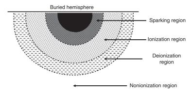
Figure 11.5 Different regions of ionization as visualized in the model of Wang et al. [12]
