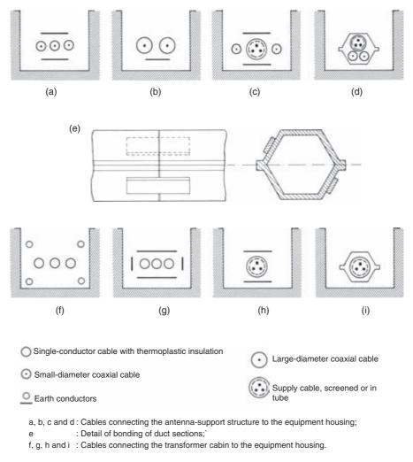
Figure 15.21 Arrangements of cables in the ducts
