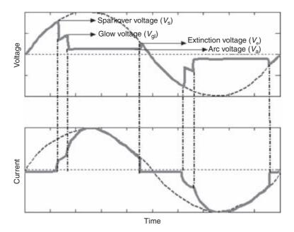
Figure 5.9 Typical response of a low-voltage gas discharge tube to an applied sinusoidal overvoltage: (a) voltage across the gas discharge tube; (b) current through the gas discharge tube
