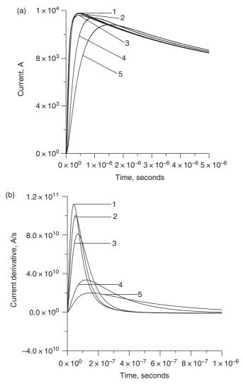
Figure 23.3 The effects of ground conductivity on the channel base current as predicted by the model of Cooray and Rakov [30] for (1)  $0.01 \text{ Sm}^{-1}$ , (2)  $0.002 \text{ Sm}^{-1}$ , (3)  $0.001 \text{ Sm}^{-1}$ , (4)  $0.0002 \text{ Sm}^{-1}$ and (5)  $0.0001 \text{ Sm}^{-1}$ : (a) current; (b) current derivative.
