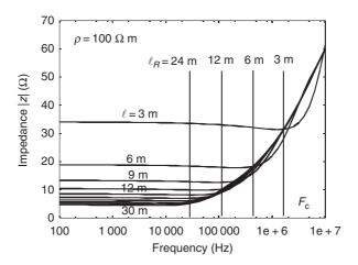
Figure 10.12 Harmonic impedance frequency dependence of horizontal wires in 100  $\Omega$  m earth
