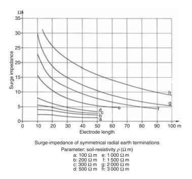
Figure 15.14 Conventional earth impedance of symmetrical radial earth termination. Parameter: soil resitivity  $\rho$  ( $\Omega$  m).
