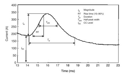
Figure 2.41 An expanded portion of the continuing current current ( $I_{CC}$ ) record of Figure 2.40 showing the definitions used in the measurement of M-current magnitude ( $I_M$ ), 10–90 per cent rise time (RT), duration ( $T_M$ ), and half-peak width ( $T_{MW}$ )
