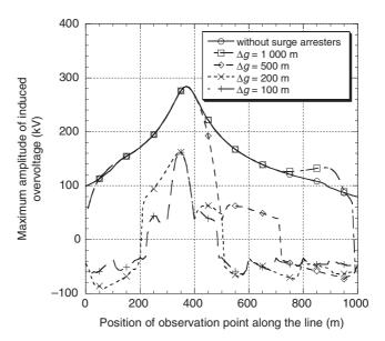
Figure 13.17 Maximum amplitude of the induced voltage along the line as a function of the spacing between two adjacent surge arresters ( $\Delta$ sa). Line configuration of Figure 13.15, stroke location 50 m from the line and 370 m from left line termination. Lossy ground  $\sigma = 0.001 \text{ S m}^{-1}$ . Lightning current: maximum amplitude 30 kA, maximum time derivative 100 kA  $\mu$ s<sup>-1</sup> (adapted from Reference 32).
