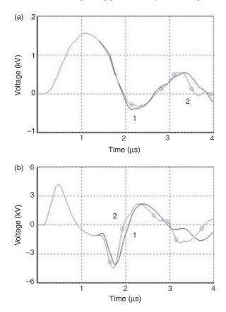
Figure 12.48 Phase-to-neutral induced voltages at point 4 of Figure 12.47 when the stroke location is in front of it, at a distance of 50 m: (a) first stroke; (b) subsequent stroke. Stroke currents depicted in Figure 12.17a. Curve 1, configuration 1; curve 2, configuration 2.
