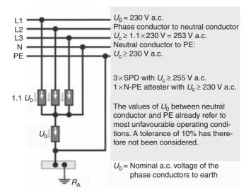
Figure 7.51 TT system (230/400 V): '3 + 1' circuit
