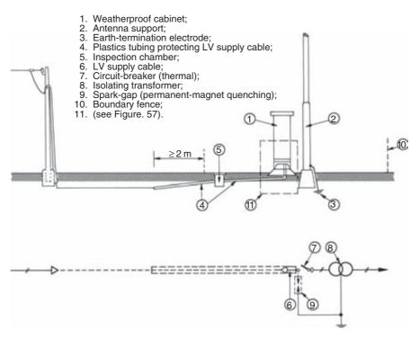
*Figure 15.23 Typical arrangement of a low-power station fed at LV and having the equipment housed in a weatherproof cabinet*
