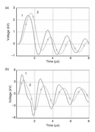
Figure 12.22 Phase-to-neutral induced voltages corresponding to the stroke currents of Figure 12.17a with different propagation velocities v: (a) first stroke; (b) subsequent stroke. Line configuration indicated in Figure 12.19. Curve 1, v = 60 per cent c; curve 2, v = 20 per cent c.
