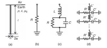
Figure 10.7 Low-current models of a vertical ground rod: (a) physical situation, (b) low-frequency equivalent circuit, (c) high-frequency lumped RLC circuit, (d) high-frequency distributed parameters circuit
