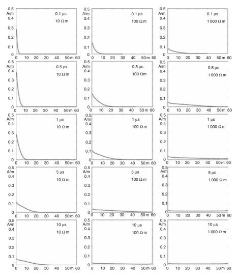
Figure 10.20 Temporal and spatial distribution of the leakage current along a 60-m-long horizontal wire as a response to an injected doubleexponential  $(T_1/T_2 = 1 \ \mu s/50 \ \mu s)$  current pulse with a peak value 1 kA, at 0 m end in earths with resistivities of 10, 100 and 1 000  $\Omega$  m
