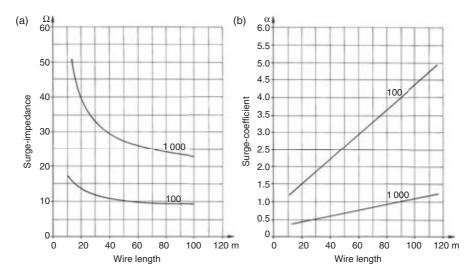
Figure 15.2 (a) Conventional earth impedance of a buried wire as a function of its length. Impulse current: 5 kA,  $7/17 \mu s$ . Parameters soil resistivity ( $\Omega m$ ). (b) Surge coefficient of a buried wire as a function of its length. Parameters soil resistivity ( $\Omega m$ ).
