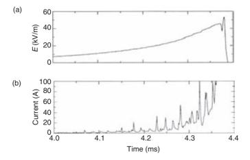
Figure 3.6 (a) Electric field measured 50 m from the lightning attachment point and (b) current produced by the upward connecting positive leader from the grounded 50 m wire in altitude triggered lightning 9516 at Camp Blanding, Florida (adapted from Reference 30)
