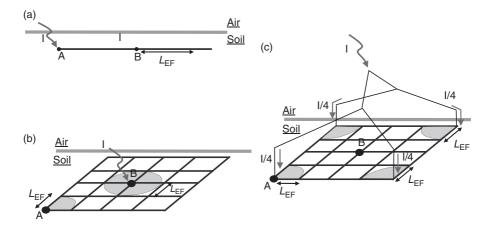
Figure 9.16 The influence of the position of the earth termination connection to buried grid on the grounding impedance: (a) horizontal electrode–earth termination at one extremity and at the midpoint; (b) grid–earth termination centre and at one corner; (c) grid: distribution of the lightning current through the four corners (adapted from Reference 2)
