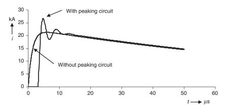
Figure 22.21 Example waveforms obtained from a peaking circuit
