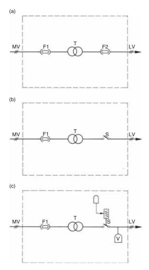
Figure 15.26 Three typical arrangements for the overvoltage protection in the step-down transformer housing
