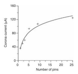
Figure 4.46 Corona current at 500 kV  $m^{-1}$  as a function of the number of needles in the cluster (adapted from Reference 136)
