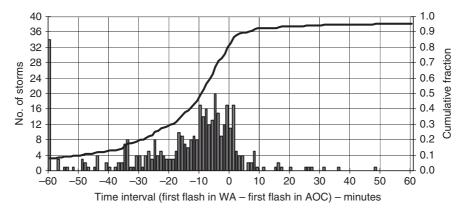
Figure 19.5 Distribution and cumulative distribution of the time interval between the first flash in the warning area (WA) and the first flash in the area of concern (AOC) for 417 storms in four locations in the United States as detected by the US NLDN
