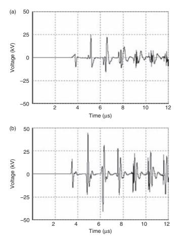
Figure 12.54 Phase-to-neutral transferred voltages at point 4 of Figure 12.47, considering the stroke currents depicted in Figure 12.17a: (a) first stroke;
