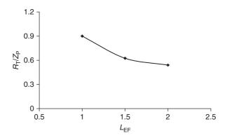
Figure 9.12 Ratio of the grounding resistance to the impulsive impedance as a function of the effective length  $L_{EF}$  (1 000  $\Omega$ m soil;  $\varepsilon_r = 10$ ; current wave,  $1/50 \ \mu$ s) (adapted from Reference 19)
