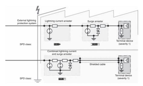
Figure 7.37 SPD combination for the protection of IT equipment
