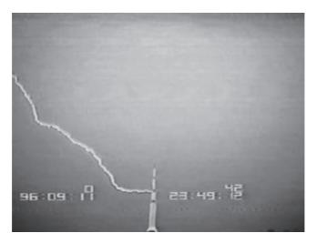
Figure 4.7 Photograph showing a lightning flash striking a point below the top of CN tower in Canada (photograph courtesy of Prof. A.M. Hussein)
