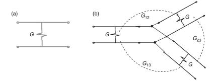
Figure 9.4 Simplification of the equivalent circuit configuration for low-frequency conditions: (a) single grounding element; (b) a set of grounding elements represented with their conductive mutual effects (adapted from Reference 1)
