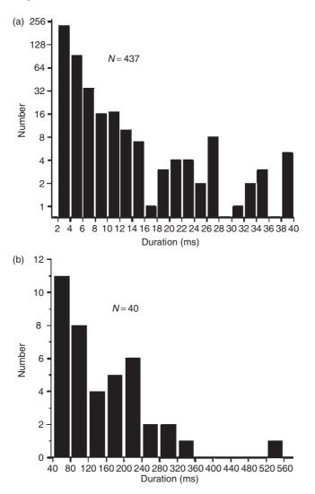
Figure 2.37 Histogram of very short continuing current durations observed by Saba et al. [25]: (a) duration below 40 ms and (b) duration above 40 ms (from Reference 24)
