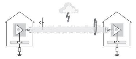
Figure 7.18 No shield connection: no shielding from capacitive/inductive couplings
