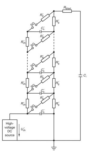
*Figure 22.5 Circuit design of a multistage impulse generator*
