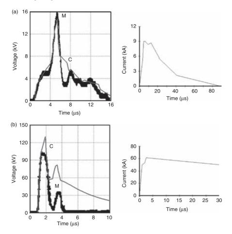
Figure 12.14 Measured (M) and calculated (C) lightning induced voltages and corresponding stroke current waveforms: (a) case 81-02 [97]; (b) case 86-03 [99] (adapted from Reference 56)
