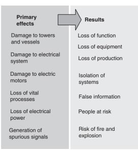
Figure 17.3 Primary effects of direct lightning incidence in offshore oil installations (OOIs)
