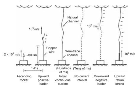
Figure 3.1 Sequence of events (except for the attachment process [25]) in classical triggered lightning. The upward positive leader (UPL) and initial continuous current (ICC) constitute the initial stage (IS) (adapted from Reference 15).
