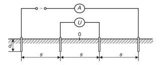
Figure 6.32 Measuring earth resistivity
