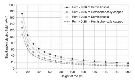
Figure 4.16 Background leader inception electric fields of a lightning rod computed with the critical radius concept for a semi-ellipsoidal rod and for a hemispherically capped rod
