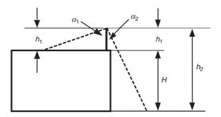
Figure 6.7 Volume protected by a vertical air-termination rod above a roof surface.  $h_1$  is the physical height of the air-termination rod. The protective angle  $\alpha_1$  corresponds to the height  $h_1$  above the roof surface to be protected, and the protective angle  $\alpha_2$  corresponds to the height  $h_2 = h_1 + H$ , the ground being the reference plane.
