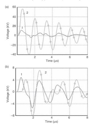
Figure 12.25 Induced voltages at the point closest to the stroke location: (a) phase-to-earth; (b) phase-to-neutral. Curve 1, situation indicated in Figure 12.19a (base case); curve 2, situation indicated in Figure 12.23.
