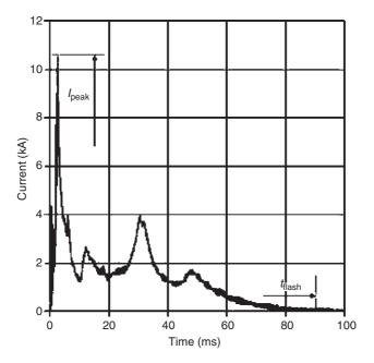
Figure 2.31 Example of a current waveform of a positive upward-initiated lightning discharge (from Reference 110)
