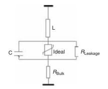
Figure 5.11 Equivalent circuit model of a varistor
