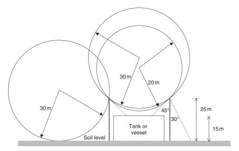
Figure 17.1 Rolling sphere method and protective angle method for the protection of tanks and vessels in an isolated external lightning protection system (ELPS). The protective angle is 45° in the bounded space of two overhead ground wires and 30° elsewhere (dashed lines). The diameter and height of the tank are 30 and 15 m, respectively. The height of the masts is 25 m.
