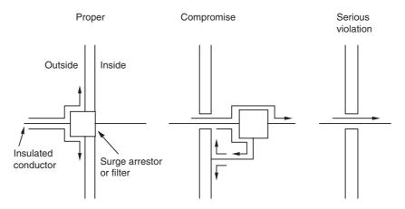
Figure 5.7 Insulated conductors or conductors that cannot be grounded (e.g. power, communication and data cables)
