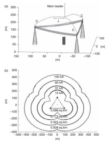
Figure 16.3 Simulation results for the protection scheme for Indian satellite launch pad-I [26]: (a) stroke interception ( $C \rightarrow$  connecting leaders and  $J \rightarrow$  final jump); (b) zone of protection for different stroke currents along with corresponding protected area
