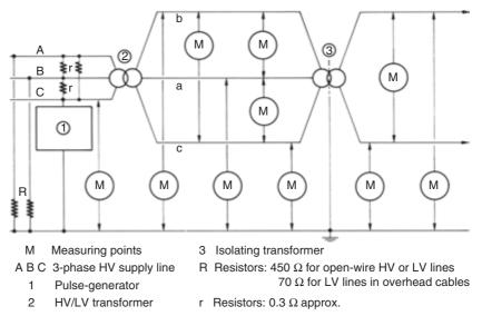
Figure A15.2 Measurement of overvoltages transferred from the power supply line
