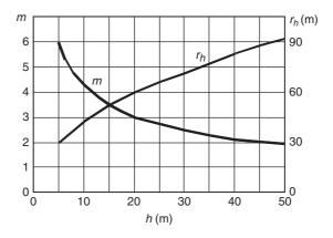
Figure 8.3 Dependence of m and r<sub>h</sub> on the structure height h
