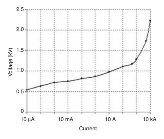
Figure 12.46 V/I characteristic of the secondary MOV arresters
