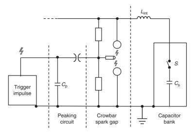
Figure 22.16 Three-electrode crowbar spark gap
