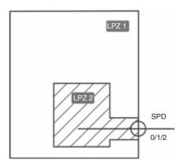
Figure 7.36 Only one SPD (0/1/2) required (LPZ 2 integrated in LPZ 1)
