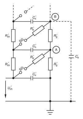
*Figure 22.6 Firing of a multistage impulse voltage generator*
