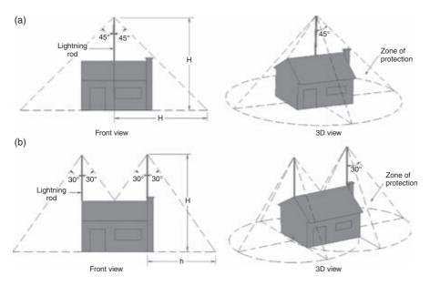
Figure 4.2 Protective angle method for the protection of a common house for an angle of (a)  $45^{\circ}$  and (b)  $30^{\circ}$
