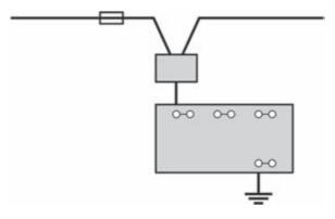
Figure 7.56 Principle of 'two-conductor terminals' (TCT): illustration of a single-pole unit
