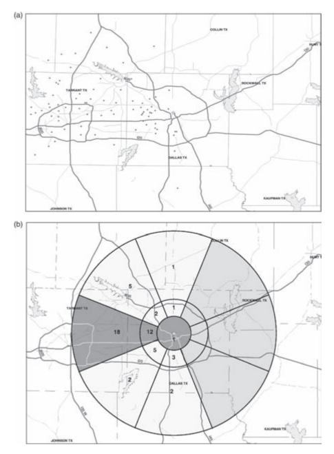
Figure 19.3 (a) Lightning locations determined by the US NLDN over a 15-min period. Map background is of northern Texas, USA (b) Representation of the same information by an application receiving information from a single-point LF/VLF lightning sensor.
