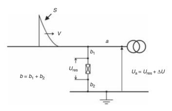
*Figure 13.8* Sketch of the protection scheme of a MV transformer directly connected to an overhead line. The protective device limits the voltage at its terminals to the protective level U<sub>res</sub> (adapted from Reference 49).
