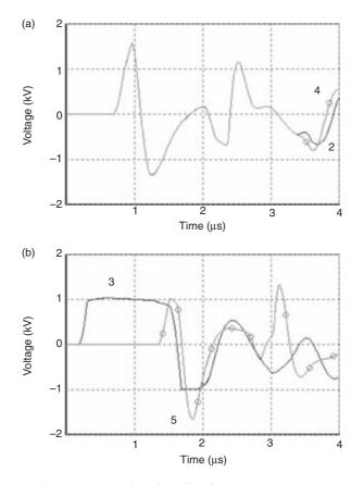
Figure 12.49 Phase-to-neutral induced voltages at points 2, 3, 4 and 5 of Figure 12.47 considering the typical subsequent stroke current depicted in Figure 12.17a: (a) points 2 (curve 2) and 4 (curve 4); (b) points 3 (curve 3) and 5 (curve 5). Configuration 2 (arresters only at the transformer terminals).
