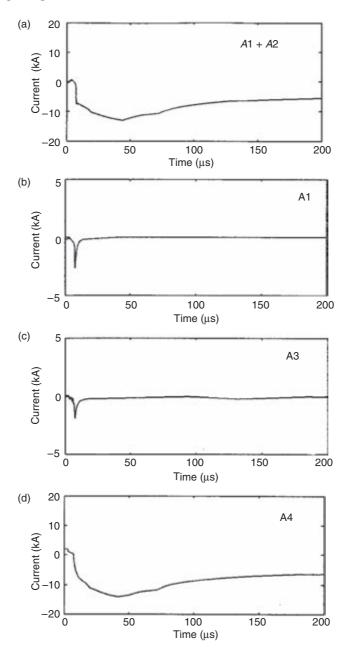
Figure 3.38 Current versus time waveforms for Flash 9706, displayed on a 200  $\mu$ s scale: (a) injected lightning current; (b) current to ground at node A (lightning protective system ground, 1 550  $\Omega$ ); (c) current to ground at node B (power system ground, 590  $\Omega$ ); (d) current entering the test house's electrical circuit (adapted from Reference 114)
