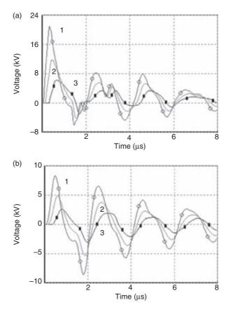
Figure 12.26 Induced voltages at the transformer LV terminals for different distances d between the line and the lightning strike point: (a) phase-to-earth; (b) phase-to-neutral. Curve 1, d = 25 m; curve 2, d = 50 m (base case); curve 3, d = 100 m.
