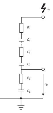
Figure 22.27 Damped capacitive impulse voltage divider
