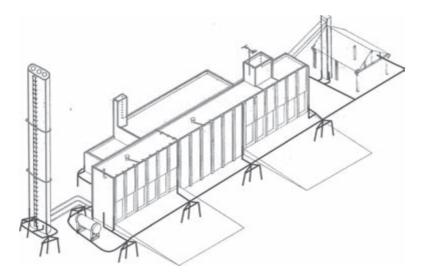
Figure 6.13 External lightning protection system of an industrial plant
