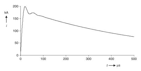
Figure 22.15 Actual waveform of an impulse current with crowbar device
