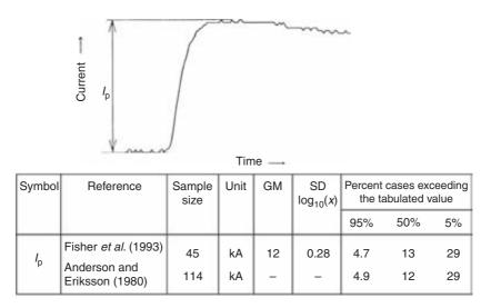
Figure 3.12 Peak current. GM is the geometric mean and SD is the standard deviation of the logarithm (base 10) of the parameter (adapted from Reference 68).
