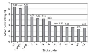
Figure 2.36 Mean peak value  $(V m^{-1})$  of return-stroke fields normalized to 100 km versus stroke order. Results are based on negative cloud-to-ground flashes observed in Brazil (from Reference 114).
