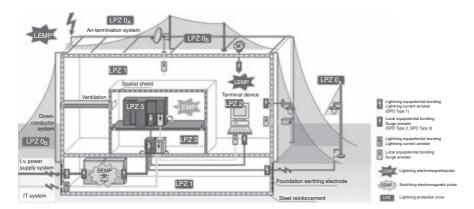
Figure 7.13 Concept of the lightning protection zones
