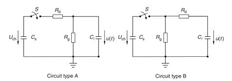
Figure 22.4 Basic circuit diagrams for impulse voltage generators
