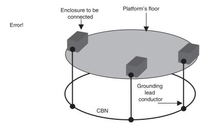
Figure 17.4 Radial connection from enclosures to the nearest CBN (equipotencial ring) of the platform's floor or level. The leads must follow the shortest distance, avoiding any abrupt turns.
