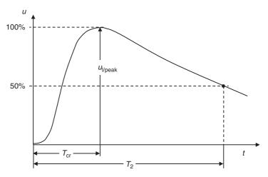
Figure 22.1 General shape and definitions of the standard switching impulse voltage  $250/2500 \ \mu s$
