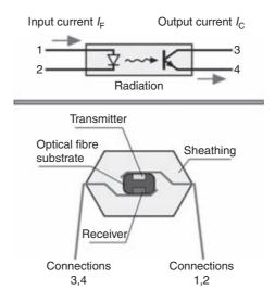
Figure 7.84 Schematic of an optocoupler
