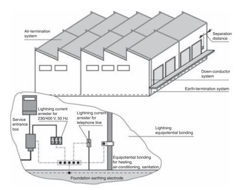
Figure 7.10 Lightning protection system
