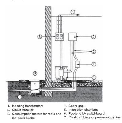
Figure 15.25 Power supply protection arrangements for a station comprising a conventional equipment building
