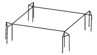
Figure 6.28 Ring conductor with triangular-prismatic vertical arrangements
