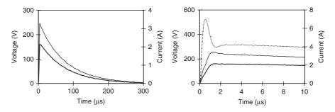
Figure 9.6 Typical result: measured current (thin line) and grounding potential rise (thick line) waves. Dashed line: voltage at the generator output – current:  $1.2/54 \ \mu s$  – soil: 116  $\Omega m$  – 3 m vertical rod – rod radius: 0.7 cm (adapted from Reference 7).
