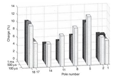
Figure 3.36 Percentage of total charge transferred to ground at different poles, calculated at three different instants of time (100 µs, 500 µs and 1 ms from the beginning of the return stroke) for stroke 1 of flash 0036 (adapted from Reference 107)
