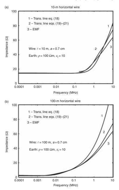
Figure 10.9 Comparison of results for harmonic ground impedance of horizontal wires for (1) transmission line equation (10.18), (2) transmission line equations (10.19) to (10.21), (3) the electromagnetic field approach [26] in (a) a 10-m horizontal wire and (b) a 100-m horizontal wire
