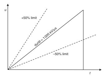
Figure 22.3 General shape and definitions of the steep front voltage waveform
