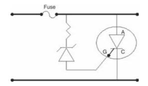
Figure 5.13 Basic thyristor crowbar circuit
