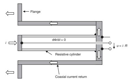
Figure 22.28 Principle of a tubular shunt
