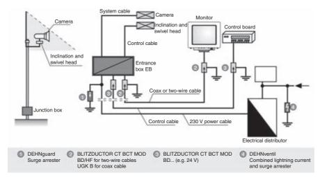
Figure 7.96 Video surveillance system: lightning and surge protection
