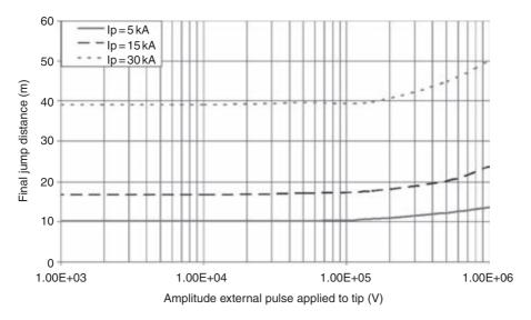
*Figure 4.42* Simulated final jump (interception) distance as a function of the amplitude of the external square voltage pulse applied to the tip of a lightning rod. Prospective return stroke peak currents of 5, 10 and 30 kA are considered (adapted from Reference 82).
