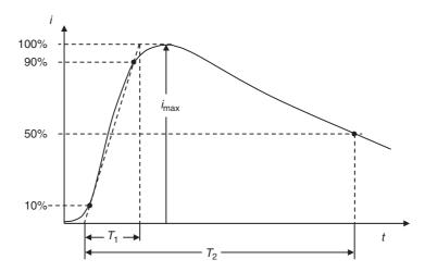
Figure 22.8 Definition of impulse current waveform parameters
