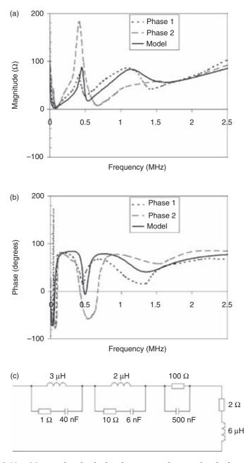
Figure 12.10 Measured and calculated input impedances of each phase of a 90 m<sup>2</sup> residential apartment (TN system) as function of frequency and corresponding equivalent circuit: (a) input impedance (magnitude); (b) input impedance (phase); (c) equivalent circuit (adapted from Reference 41)
