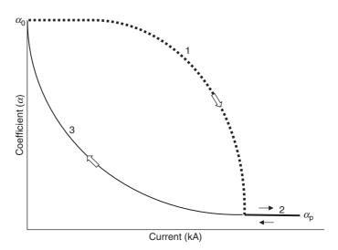
Figure 11.6 Schematic description of the way in which the coefficient α, one of the model parameters in the model of Wang et al. [12], varies as a function of current. The three regions 1, 2 and 3 are described by equations (11.29), (11.30) and (11.32), respectively.
