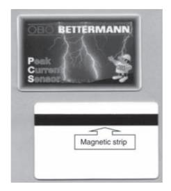
*Figure 14.25 Magnetic strip card for registering peak lightning current (photo by the author)*
