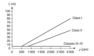
Figure 6.25 Minimum length of an earth electrode according to the class of LPS
