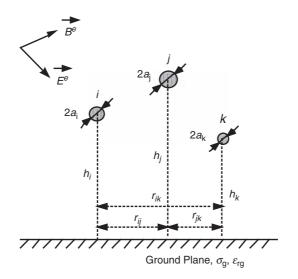
*Figure C13.1 Cross-sectional geometry of a multiconductor line in the presence of an external electromagnetic field*
