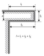
Figure 6.14 Isolation of external LPS, separation distance s on a loop in a down-conductor
