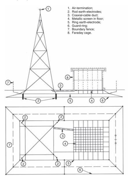
Figure 15.12 Typical earthing for a station having an autonomous power supply
