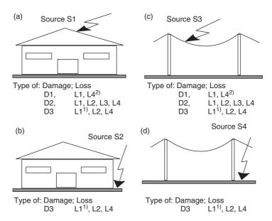
Figure 8.9 Sources of damage (S1, S2, S3, S4), types of damages (D1, D2, D3) and loss (L1, L2, L3, L4) depending on the strike point; 1) for structures where internal system failure immediately endanger human life; 2) for properties where animals may be lost
