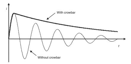
Figure 22.14 Principle of an impulse current generator
