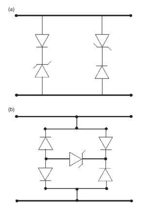
Figure 5.12 Two techniques for reducing the effective shunt capacitance of the avalanche diode
