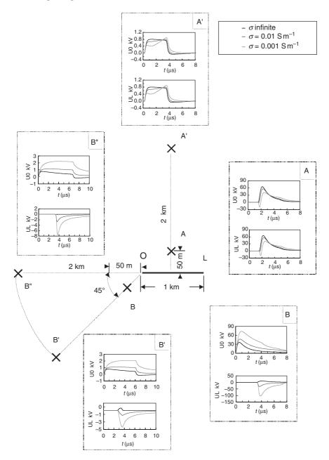
Figure 13.4 Effects of ground resistivity and position of the stroke location with respect to the line on the amplitude and waveshape of lightninginduced voltages. Solid line, perfect ground; dashed line, ground conductivity 0.01 S m<sup>-1</sup>; dotted line, ground conductivity 0.001 S m<sup>-1</sup> (adapted from Reference 43).
