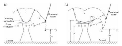
Figure 4.5 Sketch of a power transmission line and the lightning exposure arcs of the conductors according to the electro-geometrical method (EGM). This example shows a transmission line with (a) expected shielding failures and (b) perfect lightning performance.
