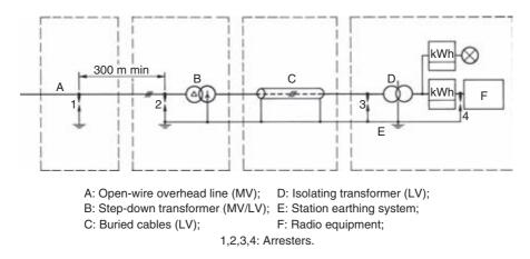
Figure 15.22 Placing of arresters in a station supply at HV by an overhead line
