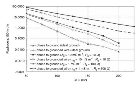
Figure 13.22 Comparison between phase-to-ground and phase-to-grounded-wire flashover rate curves calculated for different ground conductivity  $\sigma_g$ and grounding resistance  $R_g$ . Results were obtained by using LIOV-MC for the case of a line with a shielding wire grounded every 200 m and stroke locations spread over the indirect striking area (adapted from Reference 54).
