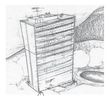
*Figure 6.12 External lightning protection system of a building*
