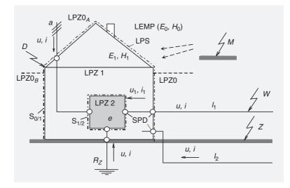
Figure 8.1 An example of the influence of lightning protection on a structure with equipment e and protection measures (screens and SPD on LPZ boundaries). D, M, W, Z, different locations of lightning strikes; SPD, surge protective devices; LPZ0, 1, 2, successive protective zones;  $S_{0/1}$ ,  $S_{1/2}$ , zone boundaries; u,  $u_1$ ,  $i_1$ , voltages and currents in entering services  $l_1$ ,  $l_2$ , a or induced; a, antenna; R, earthing; E, H, electric and magnetic fields.
