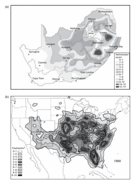
Figure 2.7 Average lightning-flash densities as measured in different regions of the world. (a) Lightning ground flash density map of South Africa [18]. (b) Lightning ground flash density map of the United States (from Reference 19).
