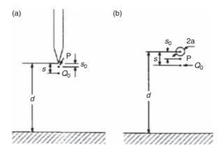
Figure 4.17 Geometry relevant to the calculation of positive leader inception according to Rizk [62] for (a) a rod-plane gap and (b) a conductor-plane gap
