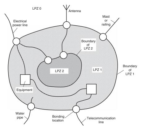
Figure 21.7 Principle of the LPZ concept
