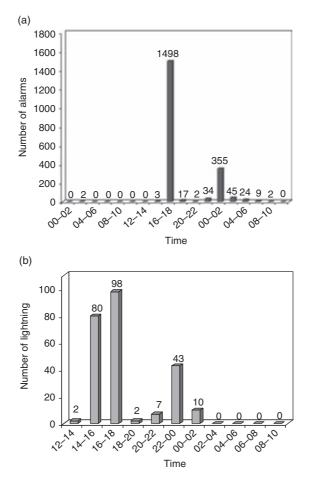
Figure 2.2 (a) Distribution of the number of false alarms caused by a thunderstorm in Malmö and Lund, Sweden on 1 July 1988. (b) The number of lightning flashes observed in the same region by the lightning-location system (modified from Reference 2).
