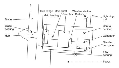
Figure 14.6 Generalized wind turbine nacelle design
