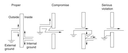
Figure 5.5 Grounding conductors (e.g. grounding of a cabinet)
