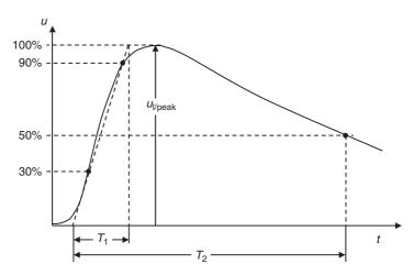
Figure 22.2 General shape and definitions of the standard lightning impulse voltage  $1.2/50 \ \mu s$
