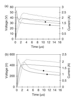
Figure 9.7 Results for a 12-m-long horizontal electrode [0.5 m deep, r = 0.7 cm; approximated value of the current wave (•) front time: 0.5 µs, 3 µs]: (a) 250  $\Omega$ m soil,  $R_{LF} = 30 \Omega$ ; (b) 3.8 k $\Omega$  m soil,  $R_{LF} = 487 \Omega$ (adapted from Reference 7)
