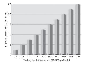
Figure 7.35 Comparison of the amplitudes of test currents waveform  $10/350 \ \mu s$ and  $8/20 \ \mu s$ , each at equal loads
