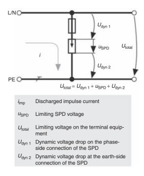
Figure 7.58 Connection of SPDs in cable branches
