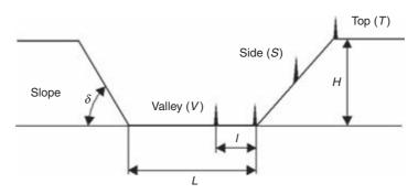
Figure 13.2 Parameters used for the evaluation of the influence of orography on the expected number of direct strokes to a MV line (adapted from Reference 19).
