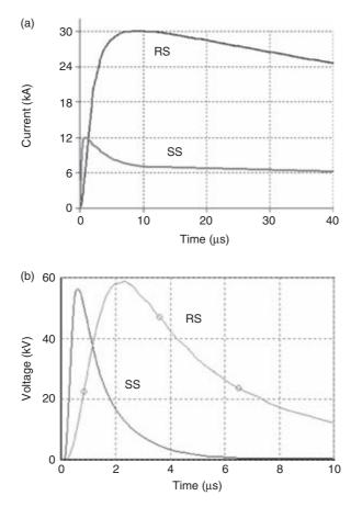
Figure 12.17 Stroke currents and corresponding induced voltages in the middle of the line shown in Figure 12.16 in the absence of the transformer and of the neutral conductor: (a) first (RS) and subsequent stroke (SS) currents waveforms; (b) induced voltages
