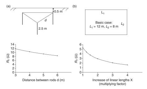
Figure 9.18 Grounding resistance as a function of covered area; 100 Ωm soil:
