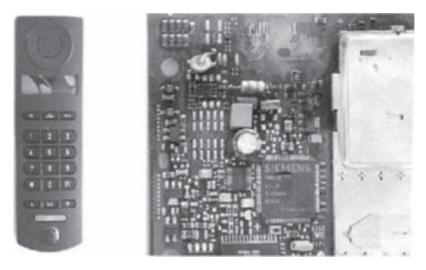
Figure 7.8 Paralysed telephone system caused by lightnings
