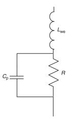
Figure 5.25 Commonly used model for resistor
