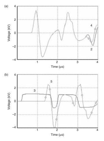
Figure 12.51 Phase-to-neutral induced voltages at points 2, 3, 4 and 5 of Figure 12.47 considering a subsequent stroke with the current waveform depicted in Figure 12.17a but with amplitude of 29.2 kA: (a) points 2 (curve 2) and 4 (curve 4); (b) points 3 (curve 3) and 5 (curve 5). Configuration 2 (arresters only at the transformer terminals).
