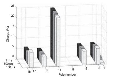
Figure 3.35 Percentage of total charge transferred through phase C arresters at different poles and terminating resistor at pole 1, calculated at three different instants of time (100  $\mu$ s, 500  $\mu$ s and 1 ms from the beginning of the return stroke) for stroke 1 of flash 0036. No measurements are available at pole 8 and pole 18 (adapted from Reference 107).
