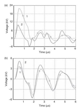
Figure 12.30 Induced voltages at the transformer LV terminals for different values of the earth resistance (Rg): (a) phase-to-earth; (b) phase-to-neutral. Curve 1, Rg =  $100 \Omega$ ; curve 2, Rg =  $5 \Omega$ .
