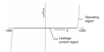
*Figure 5.10* V–I *curve of a metal oxide varistor*
