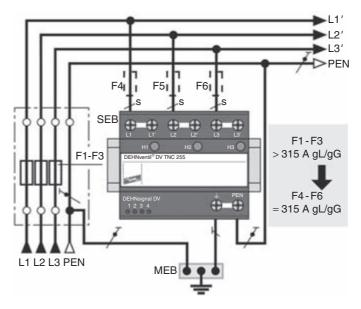
Figure 7.64 Parallel connection
