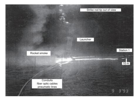
Figure 2.12 Photograph of the surface arcs emanating from the ground rod conducting a 29.6 kA rocket-triggered lightning strike to ground at Fort McClellan, Alabama [38] (from Reference 39)
