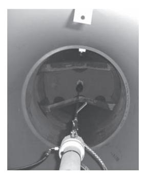
Figure 14.18 A hydraulic piston controlling a steel wire extending into the blade towards the tip air brake. A black hydraulic hose can be seen on the left side of the piston housing and on the right a flexible copper conductor connecting the steel wire and the piston housing (photo by the author).
