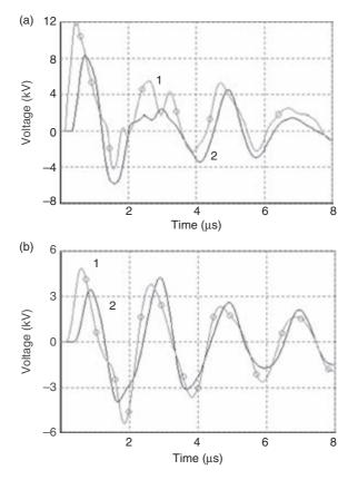
Figure 12.24 Induced voltages at the transformer LV terminals for two relative positions of the stroke location with respect to the line: (a) phase-to-earth; (b) phase-to-neutral. Curve 1, stroke location in front of the transformer (Figure 12.19, base case); curve 2, stroke location midway between the transformer and a LV power installation (Figure 12.23).
