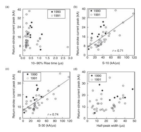
Figure 3.18 Scatterplots relating various return stroke parameters. Solid circles represent 1990 data from KSC, Florida, and open circles represent 1991 data from Fort McClellan, Alabama. (a) Current peak versus 10–90 per cent rise time. (b) Current peak versus S-10. (c) Current peak versus S-30. (d) Current peak versus half-peak width. Regression lines and correlation coefficients (t) are given in (b) and (c) (adapted from Reference 68).
