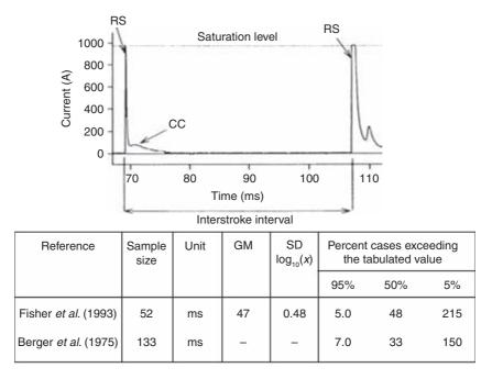
Figure 3.11 Interstroke interval. RS is the return stroke, CC the continuing current, GM the geometric mean and SD the standard deviation of the logarithm (base 10) of the parameter (adapted from Reference 68).
