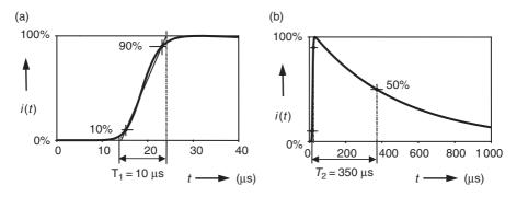
*Figure 21.1 Waveform of the first short stroke current during the rise (a) and the decay (b)*
