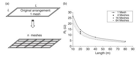
Figure 9.14 Grounding resistance of grids as a function of covered area and number of meshes: (a) square grid arrangement buried at a depth of 0.5 m;
