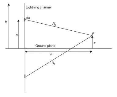
Figure 23.4 Geometry relevant to the calculation of electromagnetic fields generated by the return stroke
