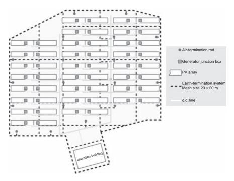
Figure 7.93 Layout of a large PV installation in an open area
