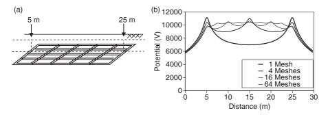
Figure 9.15 The influence of meshes on the distribution of potential on the soil: (a) line on soil surface where the distribution of electrical potential is calculated (square grid  $20 \times 20 \text{ m}^2$ ); (b) profiles of developed potential along the indicated line, soil: 500  $\Omega$ m
