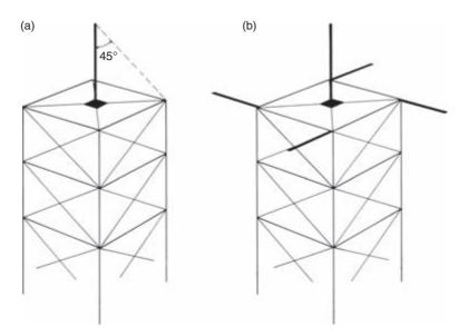
Figure 15.9 Air terminations: (a) single vertical air termination rod for low structures; (b) additional horizontal rods for structures of height greater than 20 m
