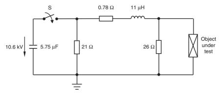
Figure 22.26 Example of a combination wave generator  $(u_{oc/max} = 10 \text{ kV}, Z_f = 2 \Omega)$
