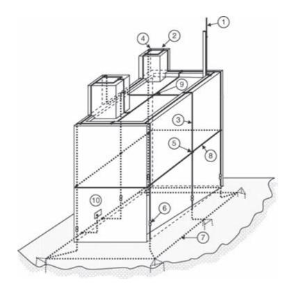
Figure 6.17 Positioning of the external lightning protection system on a low (H < 60 m) structure made of insulating material (wood, bricks, and so on). 1, Air-termination rod; 2, horizontal air-termination conductor; 3, down-conductor; 4, T-type joint; 5, cross type joint; 6, test joint; 7, ring earth electrode (type B earthing arrangement); 8, equipotentialization ring conductor; 9, flat roof with roof fixtures; 10, terminal for connecting the equipotentialization bar to the internal LPS.</li>
