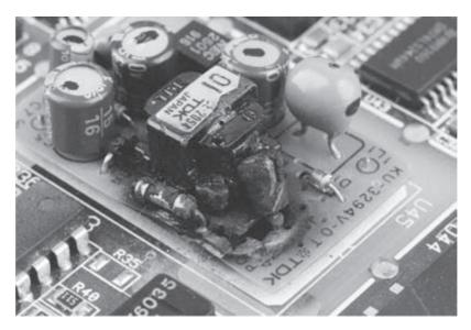
Figure 7.2 Damage caused by a surge
