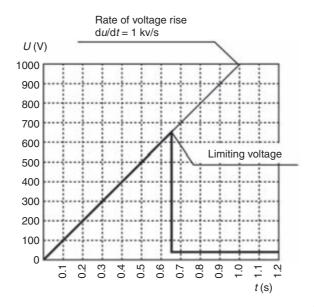
*Figure 7.79* Sparkover performance of an SPD at  $du/dt = 1 \ kV \ \mu s^{-1}$
