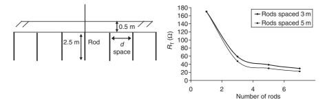
Figure 9.19 Grounding resistance as a function of the number of rods (spaced 3 and 4 m); soil: 500  $\Omega$ m
