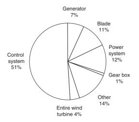
Figure 14.8 Distribution of damaged components in a total of 900 wind turbines affected by lightning in Denmark in the period 1990–1999 (from Reference 11)
