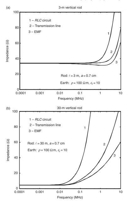
Figure 10.8 Comparison of results for harmonic ground impedance of vertical rods for (1) a lumped RLC equivalent circuit [equation (10.12)], (2) transmission line theory [equation (10.16)], (3) an electromagnetic field approach [22] in (a) a 3-m vertical rod and (b) a 30-m vertical rod
