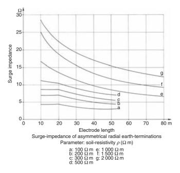
Figure 15.15 Conventional earth impedance of asymmetrical radial earth termination. Parameter: soil resitivity  $\rho$  ( $\Omega$  m).
