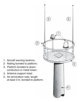
Figure 15.10 Air terminations rods on a tower platform
