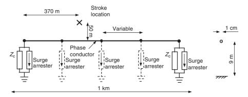
Figure 13.15 Configuration adopted to evaluate the mitigation effect of surge arresters on lightning-induced voltages. Lightning current: maximum amplitude, 30 kA maximum time derivative 100 kA  $\mu s^{-1}$  (adapted from Reference 32).
