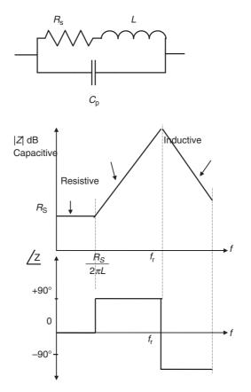
Figure 5.21 Impedance magnitude and phase of a real inductor
