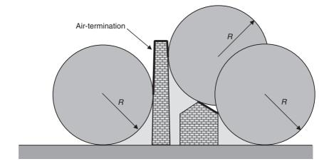
Figure 6.3 Design of an air-termination system according to the rolling sphere method
