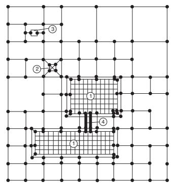
Figure 6.29 Meshed earth-termination system of an industrial plant
