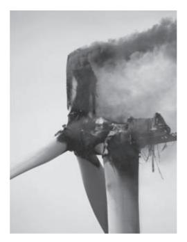
Figure 7.5 Lightning damage at a windpower station
