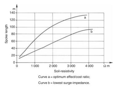
Figure 15.16 Minimum lengths of radial earth-electrodes for soil of high resistivity
