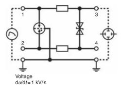
*Figure 7.78* Test arrangement for determining the limiting voltage at a rate of voltage rise of  $du/dt = 1 \ kV \ \mu s^{-1}$
