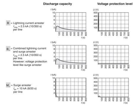
Figure 7.76 SPD classification (example: BLITZDUCTOR CT)
