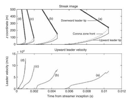
Figure 2.19 Simulated streak image and variation of the upward-connecting leader speed for different values of the downward leader velocities: (a)  $8 \times 10^4 \text{ m s}^{-1}$ , (b)  $2 \times 10^5 \text{ m s}^{-1}$ , (c)  $5 \times 10^5 \text{ m s}^{-1}$  and (d)  $1 \times 10^6 \text{ m s}^{-1}$  (from Reference 67)
