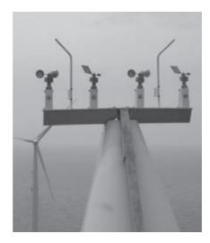
Figure 14.22 Meteorological instruments on an offshore wind turbine protected with lightning air terminals (photo by the author)
