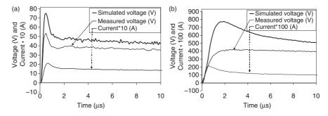
Figure 9.9 Measured voltage and current waves for a 12-m-long horizontal electrode buried 0.5 m deep, with a radius of 0.7 cm: (a) low-resistivity soil ( $\sim$ 250  $\Omega$ m) and (b) high-resistivity soil ( $\sim$ 3.8 k $\Omega$ m) (adapted from Reference 14).
