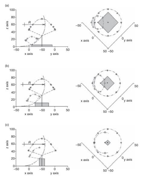
Figure 4.36 Side and top views of a square structure (a) 5 m, (b) 10 m and (c) 20 m tall protected according to the rolling sphere method (R = 60 m) with an air terminal at the centre of its roof. In all cases, the air terminal tip is located 30 m above ground [108]. The figure depicts the attractive zones corresponding to one corner and the air terminal simulated with SLIM. The dashed area in the top view corresponds to the exposure area of the corner to vertical downward stepped leaders.
