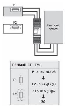
Figure 7.70 Backup protection for SPD class III (DEHNrail)
