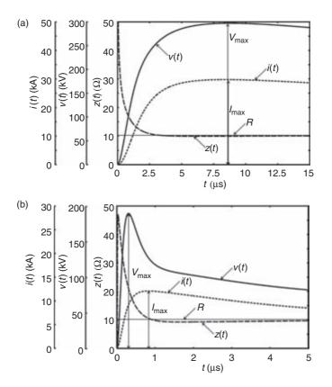
Figure 10.18 Lightning current pulse i(t), transient voltage v(t) and ground impedance of a 12-m ground rod: (a) response to a typical first stroke current pulse; (b) response to a typical subsequent stroke current pulse
