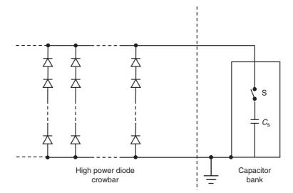
Figure 22.17 High-power diode crowbar device
