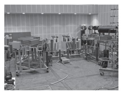
Figure 22.10 Example of an impulse current generator
