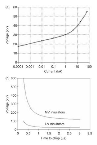
Figure 12.39 Characteristics of the surge arresters and insulators relevant to the simulations presented in Figure 12.37: (a) non-linear V/I characteristic of the ZnO MV surge arresters; (b) V/t characteristic curve for MV and LV insulators
