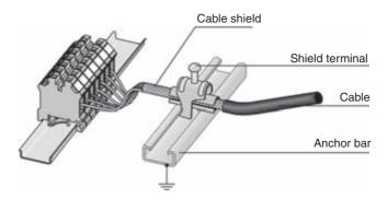
Figure 7.21 Shield connection
