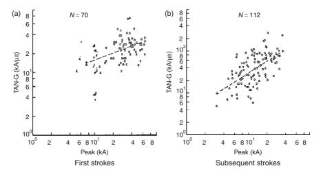
Figure 2.23 Correlation between the peak current and peak-current derivatives for first and subsequent strokes as observed by Anderson and Eriksson for the data of Berger et al. [78]
