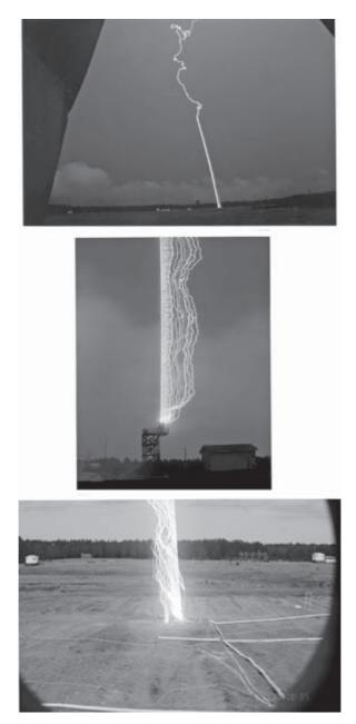
Figure 3.2 Photographs of lightning flashes triggered at Camp Blanding, Florida. Top, a distant view of a strike to the test runway; middle, a strike to the test power system initiated from the tower launcher; bottom, a strike initiated from the underground launcher at the centre of a  $70 \times 70 \text{ m}^2$ buried metallic grid.
