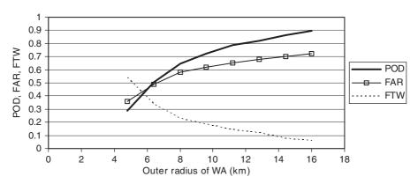
Figure 19.13 Variation of POD, FAR and FTW as a function of the outer radius of a circular WA centered on a circular AOC with a constant radius of 3 km. Analysis is a composite of several cases in the United States using data from the NLDN [35].
