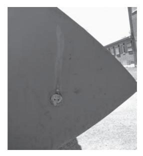
*Figure 14.17 Typical scorching of the painted surface of a blade tip on a 40-m blade where lightning has attached to the receptor (photo by the author)*
