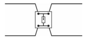
Figure 7.67 SPD with through-wiring
