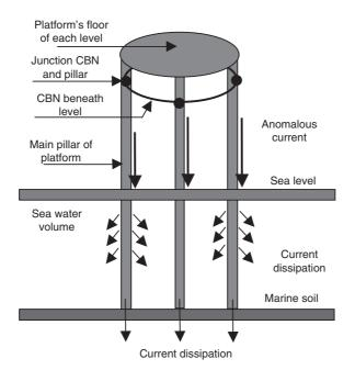
Figure 17.5 Anomalous current path from CBN (equipotential rings) and main pillars, which are considered the lowest impedance elements in OOIs of the bottom founded structure type. The current is dissipated (to some extent) in the seawater volume and (predominantly) in marine soil.
