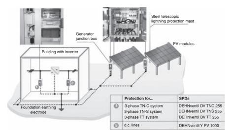
Figure 7.94 SPDs for data acquisition and evaluation
