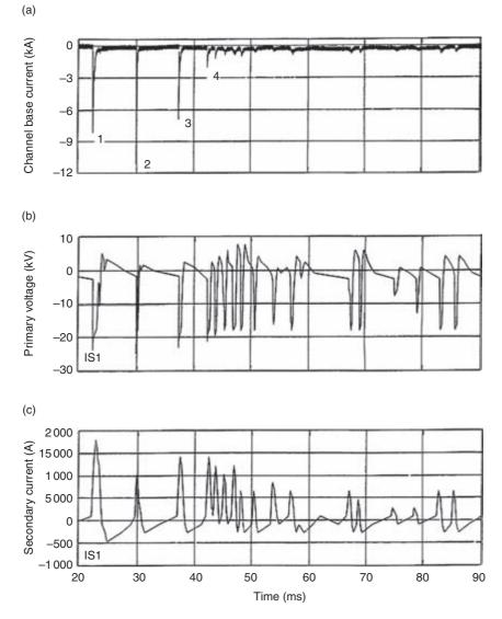
Figure 5.1 (a) Current at the channel base of a four-stroke triggered-lightning flash.
