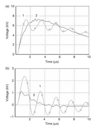
Figure 12.36 Induced voltages at the transformer LV terminals for different line configurations, considering the typical first stroke current depicted in Figure 12.17a: (a) phase-to-earth; (b) phase-to-neutral. Curve 1, rural line (Figure 12.19); curve 2, urban line (Figure 12.34).
