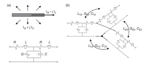
Figure 9.3 Current components in electrode and soil and the equivalent circuit for the grounding system: (a) single grounding element; (b) representation of a set of connected grounding elements with mutual effects among them (inductive, conductive and capacitive) (adapted from Reference 1)
